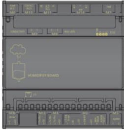
Humidifier control board
