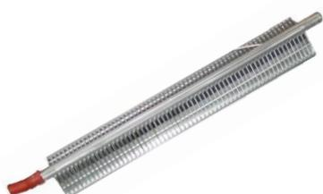
Electric heater consisting of finned aluminum elements, ensuring low surface temperature and deleting the air ionization problems. The optional is installed downstream the main cooling coil. In electric heaters with three working steps the activation is binary type.
