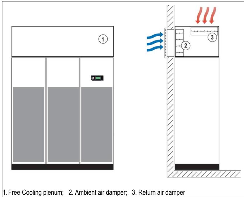
1. Free-Cooling plenum; 2. Ambient air damper; 3. Return air damper
