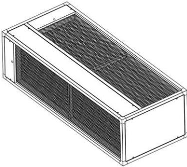
For a further energy-saving, the MEHITS conditioners are equipped with a proportional automatic free-cooling system in order to obtain free cooling when the indoor temperature is higher than outdoor one. Practically, the fresh air is used as coolant, when the outside conditions allow for this, in order to cool the ambient.
