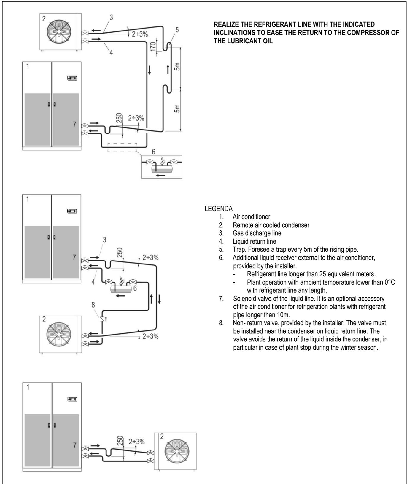
THIS DIAGRAM APPLIES TO EACH REFRIGERANT CIRCUIT OF THE UNIT.
