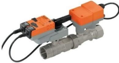
Accessory to the cooling coil and replaces the 2-way valve. Pressure-independent EPIV regulating ball valve with electronic flow control. The accessory is factory installed inside the unit and does not change its overall dimensions.
