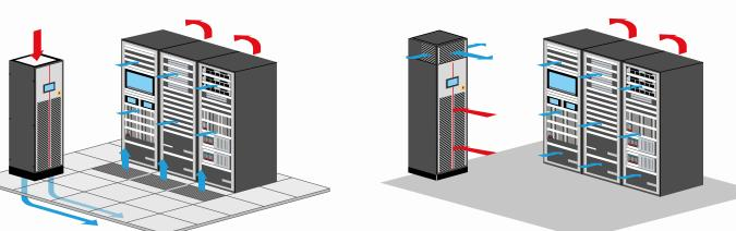
TYPICAL INSTALLATION: DATA CENTERS WITH OR WITHOUT RAISED FLOOR
