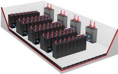
The series is particularly suitable for installation in Data Center of medium / small size with constant load, which is planned to DISPLACEMENT air delivery.
