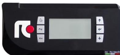
The microprocessor control system is equipped with 6 keys terminal and back lighted graphic display on which all information in different languages or easily identifiable symbols are displayed. The system disposes of a "flash" memory that preserves the information even in absence of power supply. Part of memory is dedicated to the registration of intervened events - up to 200 events.
