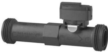
The flow meter directly measures and displays the volume of fluid transiting the unit, simplifying unit configuration during commissioning, as well as displaying the cooling capacity delivered if combined with the modulating water valve kit.
