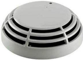
The optical smoke detector senses the presence of combustion by-products (visible smoke) and activates an alarm. The operating principle is based on the light scattering technique (Tyndall effect).
