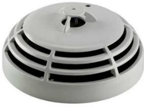
The combined smoke/fire detector senses the presence of combustion by-products (visible smoke) and/or the temperatures at which fires may start and activates an alarm. The smoke detection principle is based on the light scattering technique (Tyndall effect). The heat detector has been designed to identify temperatures at which fires may start. When the temperature exceeds the set threshold in temperature, the relay is activated to signal an alarm.
