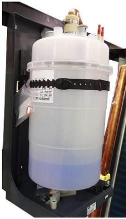
Modulating steam humidifier with immersed electrodes fitted with safety and running accessories. The accessory is factory installed and requires water filling connection. The optional accessory requires increased frame dimensions (optional) for in-row version with frontal air delivery.
